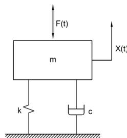
Figure 3: Model of SDOF structure upon Excitation,  $F(t)$  with Dampening and Stiffening elements
