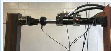
Figure 1. Set up in the Structural and Earthquake Engineering Laboratory at SFSU with servo hydraulic actuator set test performance of B-C moment.
