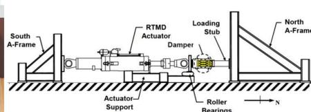
Figure 2. Servo-hydraulic Actuator Components
