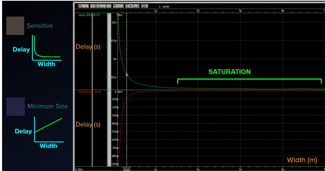
Figure 8. HSpice Delay vs Width Simulation Analysis Graph with Derivative Function
