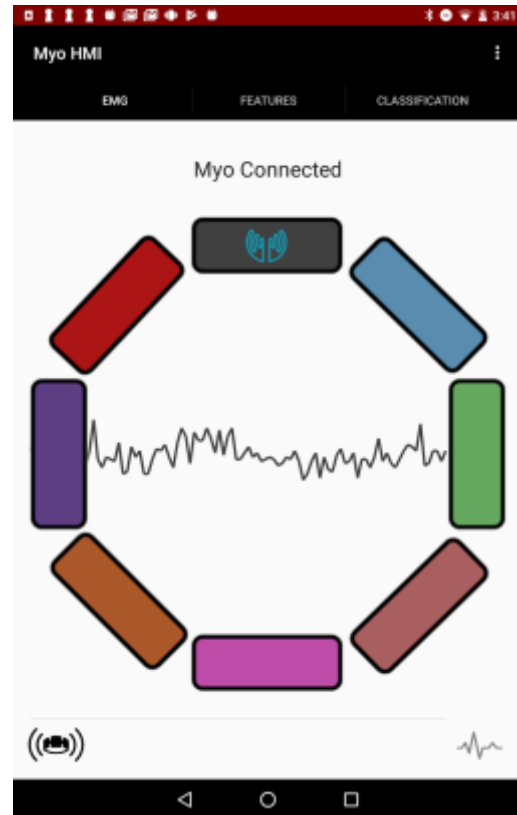
Figure 11. EMG tab in the MyoHMI application has a graph that displays raw EMG data.
