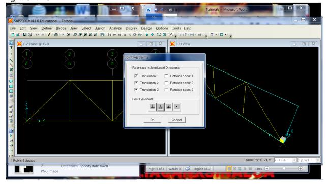
Fallow the same procedure for the other side of the truss. Select the bottom right joint, in this case we are going to assign a roller as a support for the truss. From the window show above, select the **Roller** option, which is the second from right to left.
