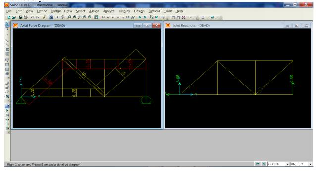
For the last part, when trying to verify whether the member is in tension or compression, just select the member you want to check, and then do a right click on it. The **Diagram Frame Window** pops up and shows the axial force. The arrows would tell whether the member is in tension  $(\leftarrow \rightarrow)$  or compression  $(\rightarrow \leftarrow)$ . Usually, reed is for compression and yellow is for tension.
