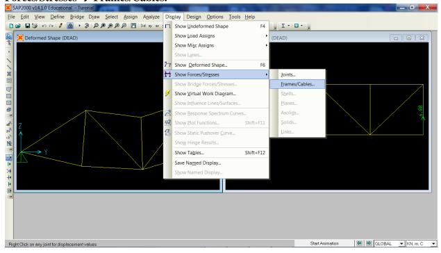
On the **Member Force Diagram Window**, click on **Axial Forces**, **Auto** and **Show Values on Diagram**. Click Ok. The forces for each member should be shown in the other window.
