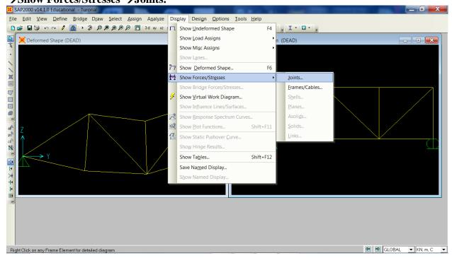
On the **Joint Reaction Forces Window** click the option **Show Results as Arrows**. Click Ok. On one of the two windows you will see the force reactions as arrows with direction and magnitude
