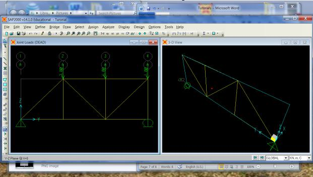
We are going to analyze each member individually, so we need to release all the truss's members (Separate them from the joints, so they can respond individually to the force being applied). Select the whole truss and then click  $Assign \rightarrow Frame \rightarrow Releases/Partial Fixity$ .
