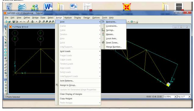
Once the **Joint Restraints Window** is up, select the **Pin** option which is the second from left to right. Click OK.
