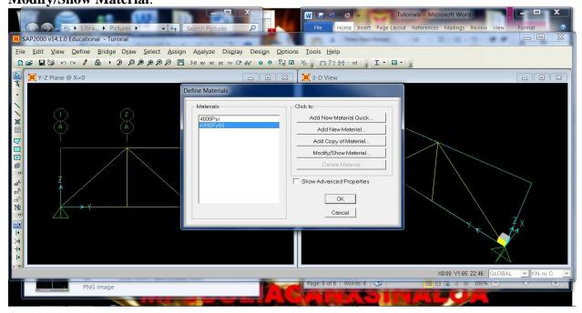
Once the Material Property Data Window is up, look for the option Weight per Unit Volume. Change this numerical value to Zero. This is because in the problem, we are not given the weight of the truss, so we are not taking it into account for our calculations, but **SAP 2000** by default takes the weight of the material, in this case **A992Fy50**, into the calculations. Click Ok.
