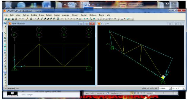
Once we have assigned the appropriate supports to our truss, we are going to define the material being use on our model. Click the option **Define** on the toolbar, and from the drop down list select **Materials.**
