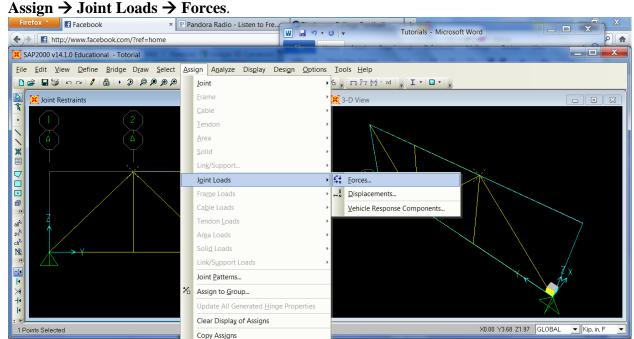
Once the **Joint Forces Window** is up, type -3 for **Force Global Z**. Fallow the same process for the other two joints, -6 for the middle top joint and -1 for the right top joint. Click Ok.
