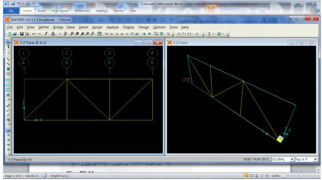
Once our model (truss) is completed, we need to assign the appropriate supports. In our problem, the truss is supported by a pin on the left side and by a roller on the right side. Select one of the bottom corner joint, in this case the left side, and from the toolbar click on **Assign**  $\rightarrow$  **Joint**  $\rightarrow$  **Restrains**.
