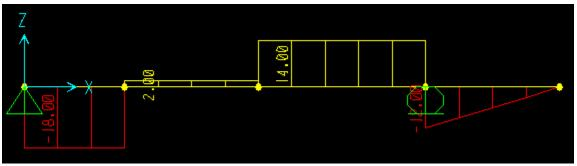
**Step 15: Display Moment Diagram:** Display → Show Forces/ Stresses → Frames/ Cables. Under Component select Moment 3-3, under Options select Show Values on Diagram and hit OK.
