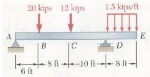
Draw the shear and bending moment diagram for
