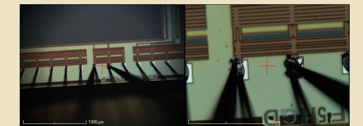
Figure 11. Section of chip being stress tested
